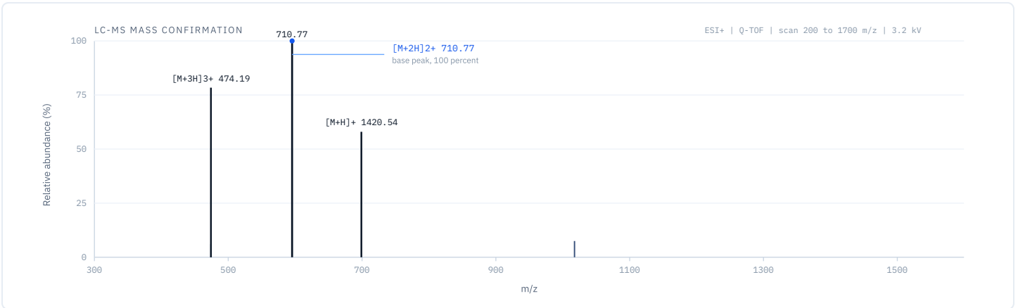
Figure 3. LC-MS mass confirmation (electrospray positive mode). Base peak [M+2H]2+ at m/z 710.77 with [M+H]+ at 1420.54, consistent with the 1419.5 Da mass of BPC-157 and confirming identity.
