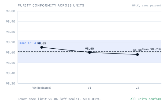
Figure 4. Purity conformity across tested units with mean and plus or minus 3 SD control band (SD 0.036%).
