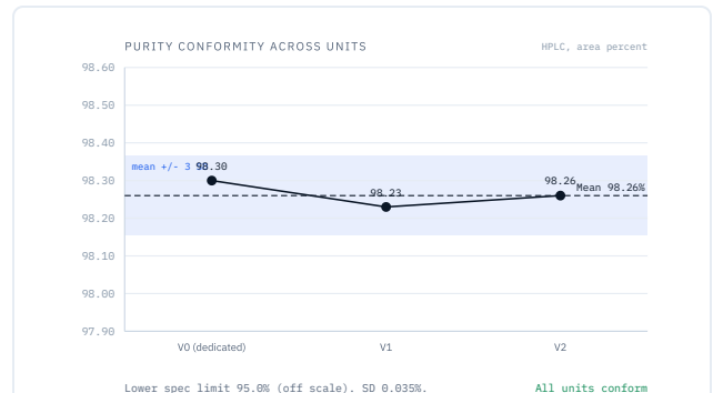
Figure 4. Purity conformity across tested units with mean and plus or minus 3 SD control band (SD 0.035%).
