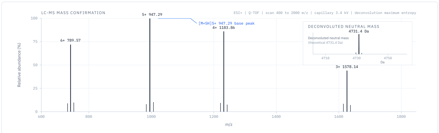
Figure 3. LC-MS mass confirmation (electrospray positive mode). The multiply-charged ion envelope from [M+3H]3+ to [M+6H]6+ deconvolutes to a neutral mass of 4731.4 Da, matching the theoretical mass of Retatrutide and confirming identity.
