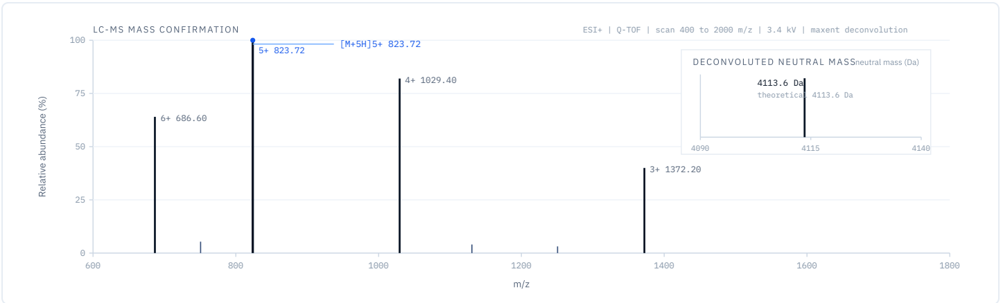
Figure 3. LC-MS mass confirmation (electrospray positive mode). The multiply-charged ion envelope from [M+3H]3+ to [M+6H]6+ deconvolutes to a neutral mass of 4113.6 Da, matching the theoretical mass of Semaglutide and confirming identity.
