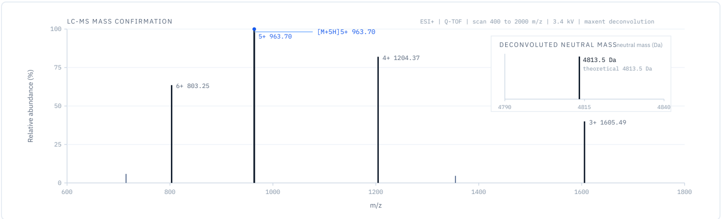
Figure 3. LC-MS mass confirmation (electrospray positive mode). The multiply-charged ion envelope from [M+3H]3+ to [M+6H]6+ deconvolutes to a neutral mass of 4813.5 Da, matching the theoretical mass of Tirzepatide and confirming identity.
